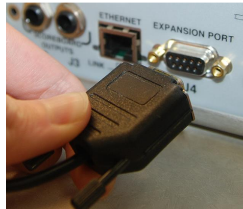
Figure 8: Wireless Photocell Connection
