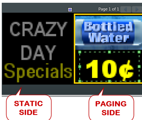
Figure 3: Static content is entered on the layout while changing content is entered in the Paging area.
