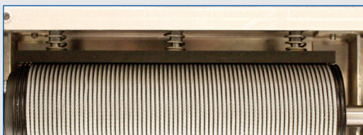
Figure 15: Drum Cable keepers
