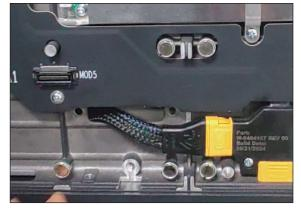
Figure 12: Install Power Input Cable
