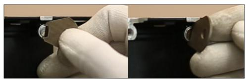
Figure 33: Using Magnetic Adjustment Tool
