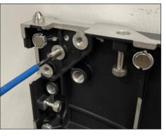
Figure 15: Adjust the Jacking Hardware
