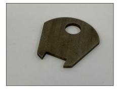
Figure 39: Magnetic Adjustment Tool
