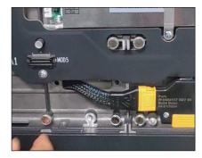
Figure 20: Install Power Input Cable
