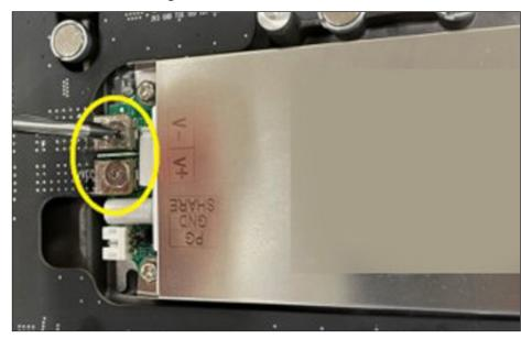
Figure 10: Remove Screws of the DC Power Connection
