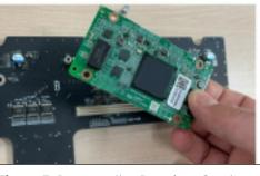
Figure 7: Remove the Receiver Card
