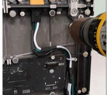
Figure 24: Secure Panel to Tube in Corners
