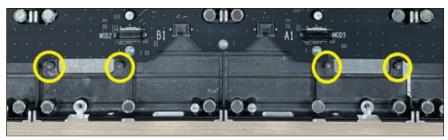
Figure 19: Remove Nuts from Cover
