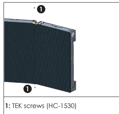
Figure 20: Install HC-1186 Screws
