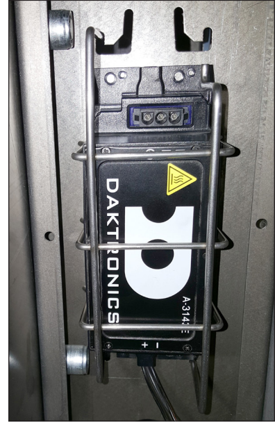
Figure 26: Controller Power Supply Mounting
