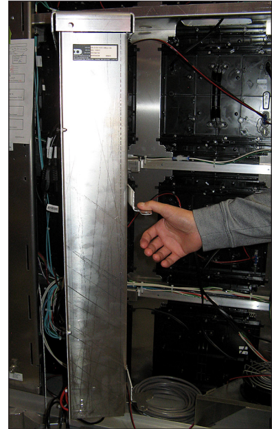
Figure 19: Swing ISP Enclosure Out of Display
