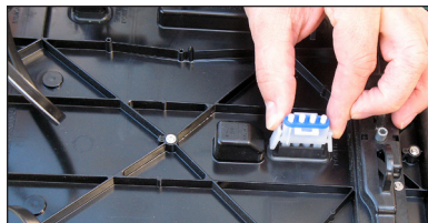
Figure 4: Remove Plug From Power Jack on Spare Module
