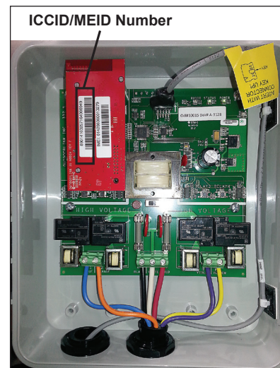
Figure 36: ICCID/MEID Number on Mezzanine Card
