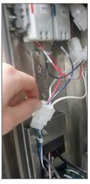
**12.** Connect female end of cable from the kit to the male connector that was just disconnected. The existing female connector can be left where it is.
