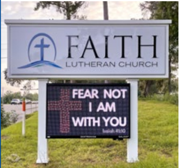
Faith Lutheran Church Tallahassee, Florida GT6x Series 108 lines x 180 columns 10 mm RGB Apogee Signs
