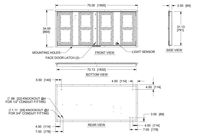
THIS IS A SINGLE FACED DROP-IN DISPLAY TO BE MOUNTED IN A RECTANGULAR OPENING IN A LARGER SIGN.
