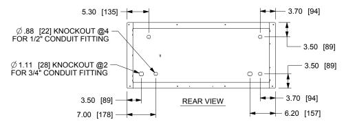
THIS IS A SINGLE FACED DROP-IN DISPLAY TO BE MOUNTED IN A RECTANGULAR OPENING IN A LARGER SIGN.
