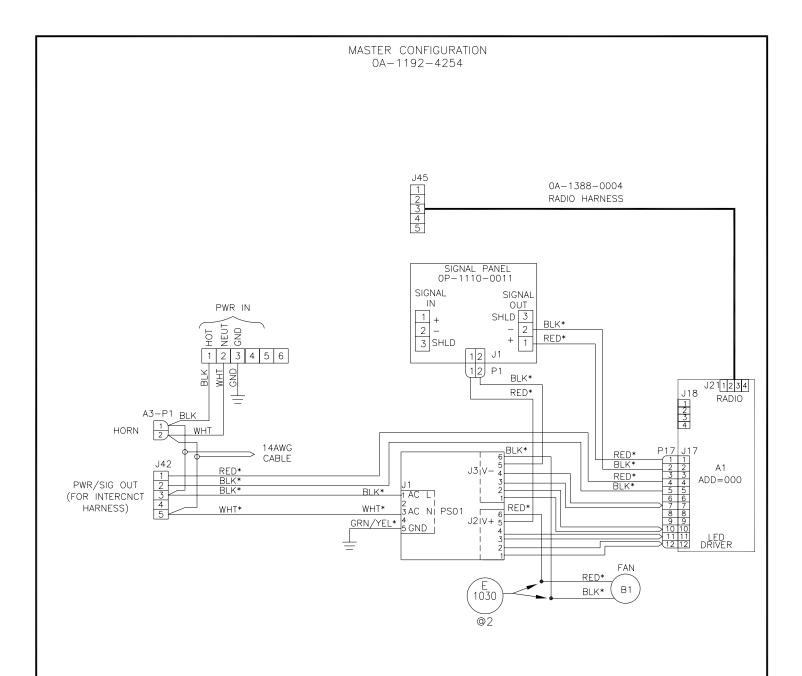
ALL CONDUCTORS ARE 14AWG EXCEPT \* INDICATES 18AWG CONDUCTORS. ALL SIGNAL WIRES IS ALSO 18AWG.
