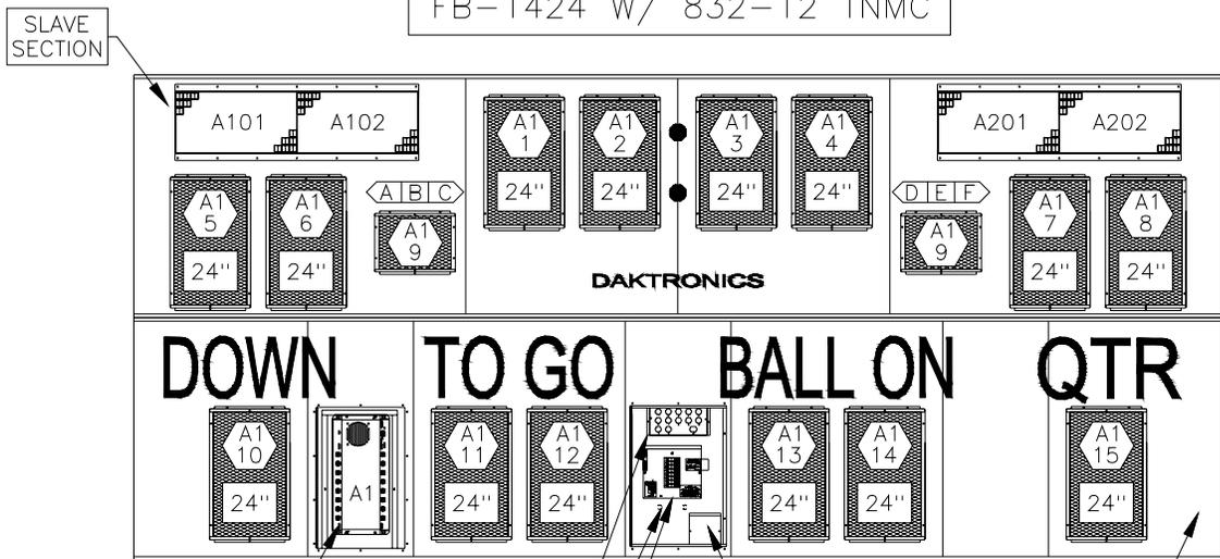
ENCLOSED 16 COLUMN LAMP DRIVER (THE COVER IS REMOVED TO SHOW THE LAMP DRIVER)      CONNECTOR PANEL FOR DIGIT HARNESS      HORN (OPTIONAL)      MASTER SECTION
