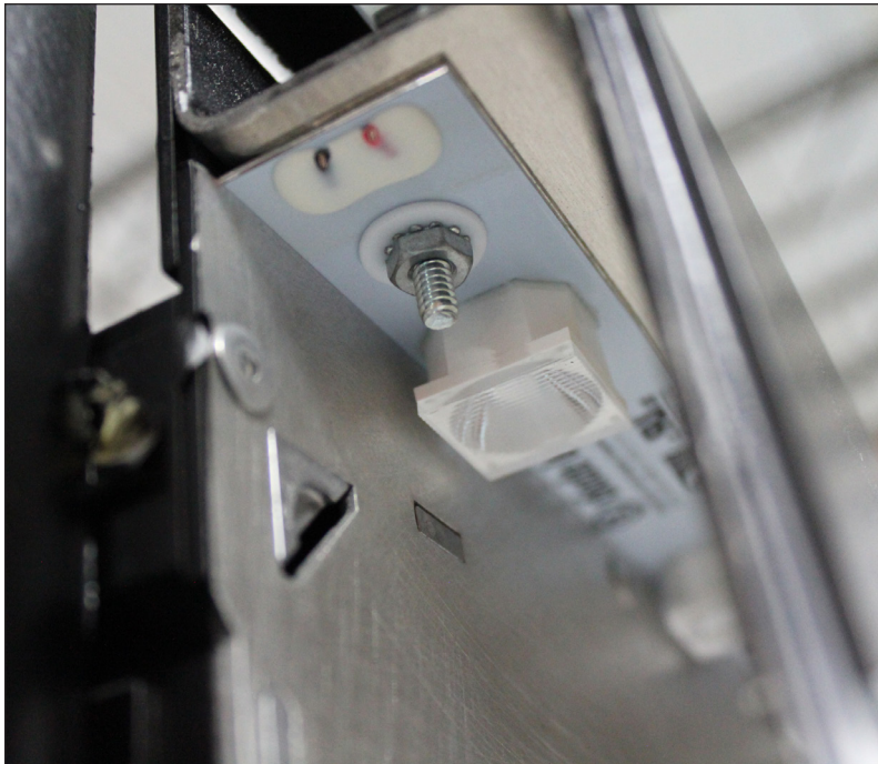
Figure 49: LED Edge Light Strip (as Viewed with Side Pads Removed)
