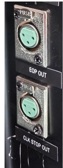
Figure 44: Light Strip Outputs
