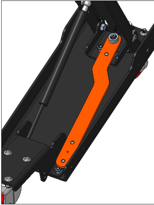
Figure 12: Caster Base Tool in Storage Position (Tool Highlighted Orange for Clarity)
