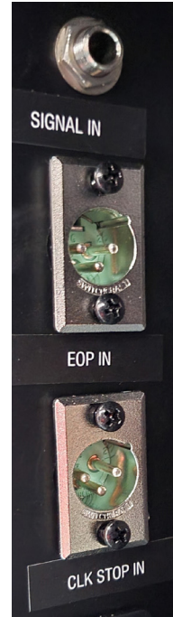
Figure 49: Light Strip Inputs
